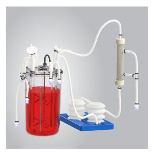
250 ml culture vessel with integrated perfusion set-up
